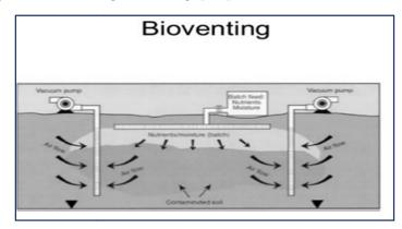
(ii) Biostimulation – It is the process where specific nutrients and electron acceptors, such as phosphorus, nitrogen, oxygen, or carbon (e.g. in the form of molasses) are injected at the site to stimulate indigenous microbial activities. [7]
